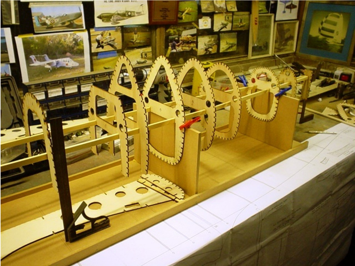
Fit formers over crutch, set up with set square to reference lines drawn on jig and glue in position.
